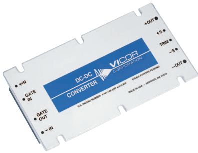
FIG 2 The first Vicor product. A megahertz-regulated 75-W dc-dc converter module with a minimum efficiency of 80% and a power density of 25 W/in 3 . It was introduced in 1984. (Image courtesy of Vicor Corp.)
