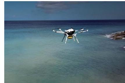
Hydrogen fuel cell-powered UAVs
