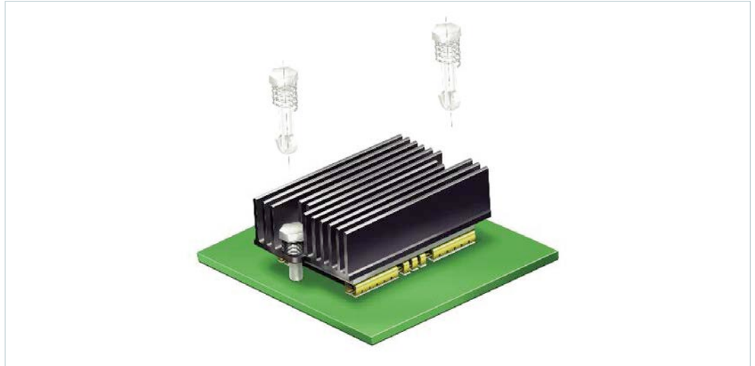
Figure 2 Mounting a Heat Sink to the BCM Increases the Effective Surface Area and Lowers R\theta_{CA} .
